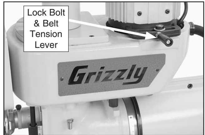
Figure 67. V-belt tension lever.
